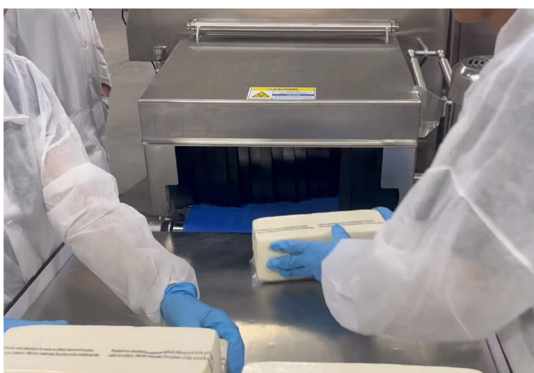
Blocks of cheese are sent through the X-ray machine for inspection. The company is also capable of operating remotely, sending X-ray machines where they are needed.
