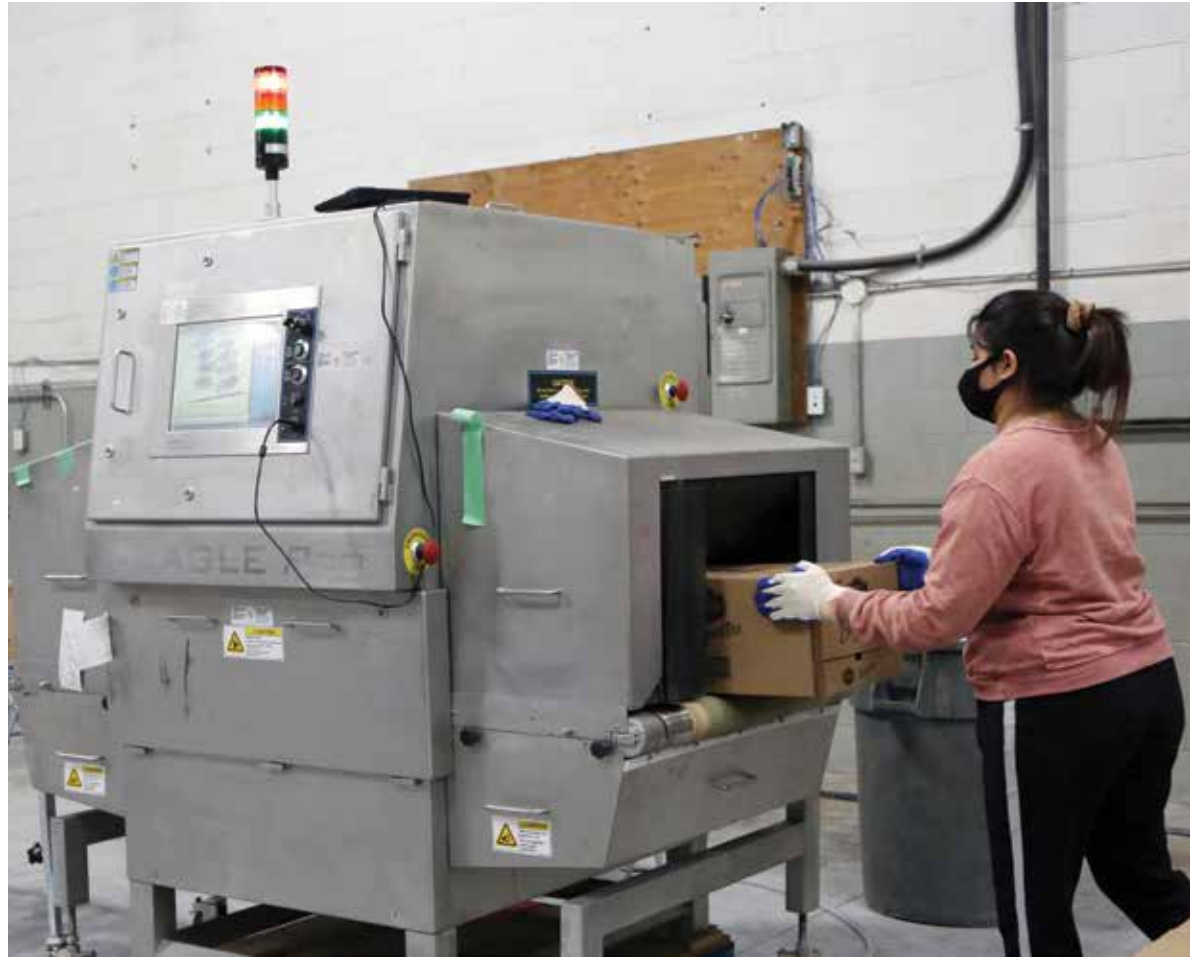
A case full of product is put through an Eagle X-Ray inspection system to find and remove small metal objects that may have found their way into the finished packages contained inside the corrugated shipping box.
